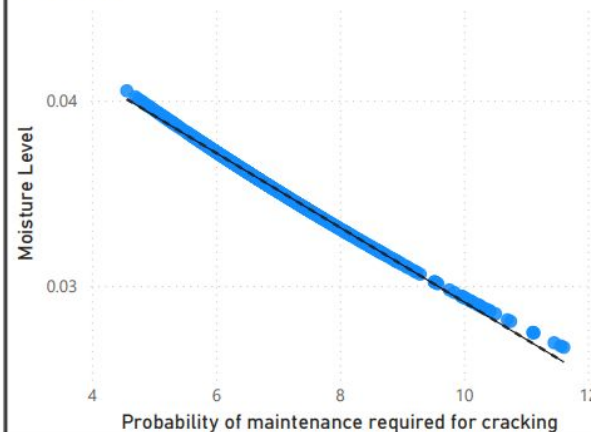
Probability of crack repairs vs moisture level | Road ID 002-0577
