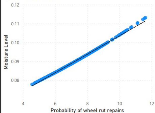
Probability of wheel rut repairs vs moisture level | Road ID 002-0577
