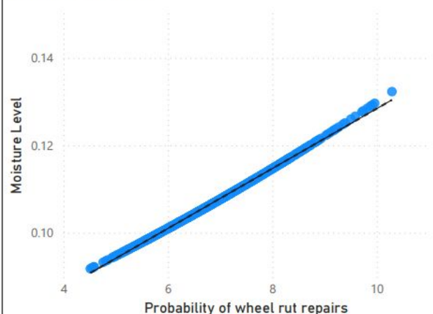
Probability of wheel rut repairs vs moisture level | Road ID 002-0544
